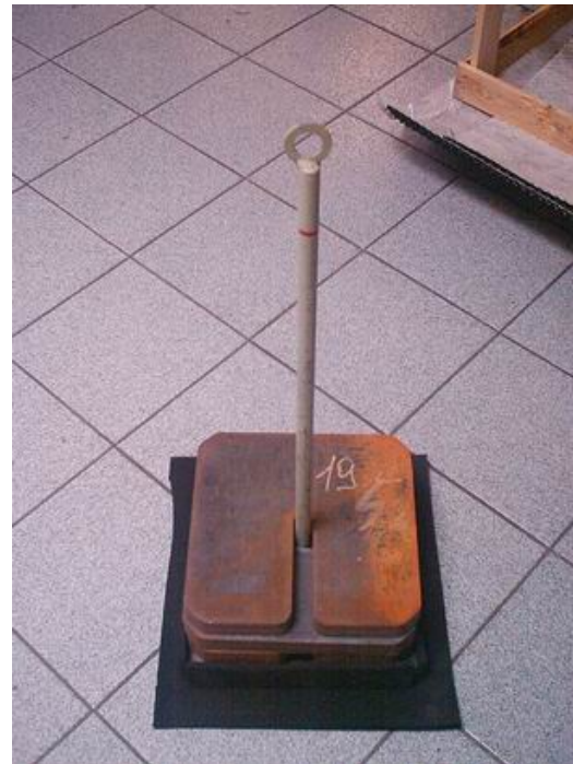
Figure 3: Testing Apparatus: the trial load
